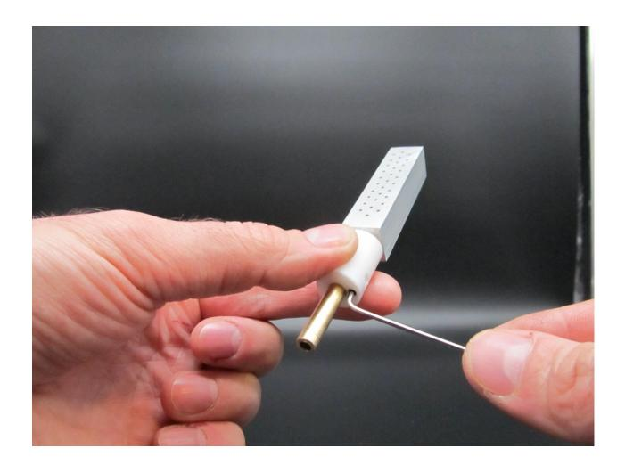
To regulate flame color (Air-fuel), you would need allen key 1.5mm! Turn the set screw on the white Teflon handle, as shown in the photo, clockwise to get yellow flame, and counterclockwise for more blue flame. Optimal flame for this burner, that have maximum height, will have blue color on the bottom and yellow on the top!
