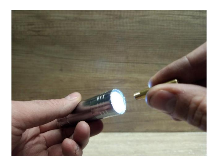
Point the gas jet thread to flashlight and look trough the jet. You should see a tiny clear hole. If you cant see the light trough the tiny hole, jet must be cleaned.
