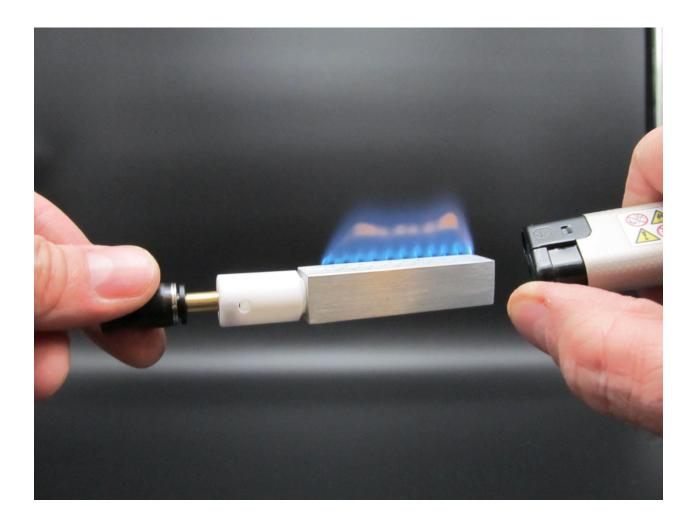
Light up the burner and get low flame at first, by slowly controling gas valve knob. Then place the burner inside your steam engine burning chamber and slowly turn the gas valve knob to get desired firepower. Be careful to not burn your hands!
